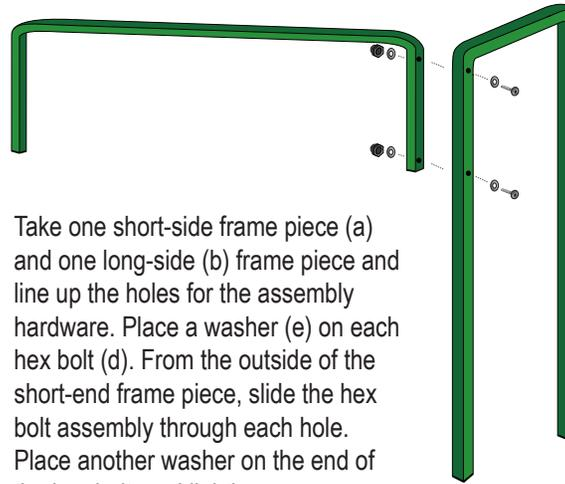
Take one short-side frame piece (a) and one long-side (b) frame piece and line up the holes for the assembly hardware. Place a washer (e) on each hex bolt (d). From the outside of the short-end frame piece, slide the hex bolt assembly through each hole. Place another washer on the end of the hex bolt, and lightly screw on a cap nut (c).
