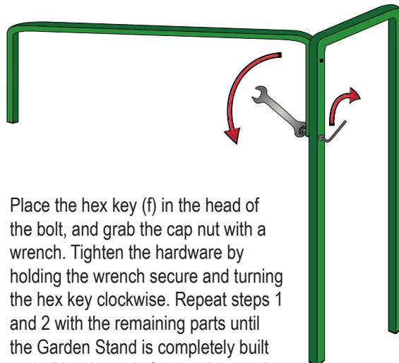
Place the hex key (f) in the head of the bolt, and grab the cap nut with a wrench. Tighten the hardware by holding the wrench secure and turning the hex key clockwise. Repeat steps 1 and 2 with the remaining parts until the Garden Stand is completely built and all hardware is fastened securely.
